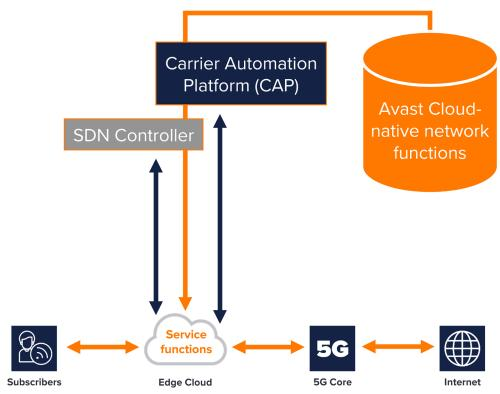
Provisioning the VNF in the 5G Edge Cloud happens when an operator's OSS/BSS indicate that a new subscriber should receive the service. The Carrier Automation Platform (CAP) then fetches the appropriate cloud-native network functions that comprise the Avast VNF and inserts them into the subscriber's service function chain in the 5G Edge Cloud. As a consequence, data traffic from and to the subscriber's endpoint passes through the Avast VNF and is checked for risk indicators.
